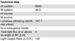
W source: Luminous efficiency (lm/W, 147.7 real value): Im in emergency mode: Total light flux at or above an angle of 90° [Lm]: Light Output Ratio (L.O.R.) 100 [%]: CRI (minimum): Colour temperature [K]: 5700 MacAdam Step: 3 Life Time LED 1: 100,000h - L90 - B10 (Ta 25°C) Lamp code: LED Number of lamps for optical 1 assembly: ZVEI Code: LED Number of optical
