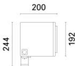
**Product code**BX14: Spotlight with bracket - Neutral White COB LED - integrated, 1-10V dimm. electronic ballast - medium optic **Attention! Code no longer in production****Technical description**
