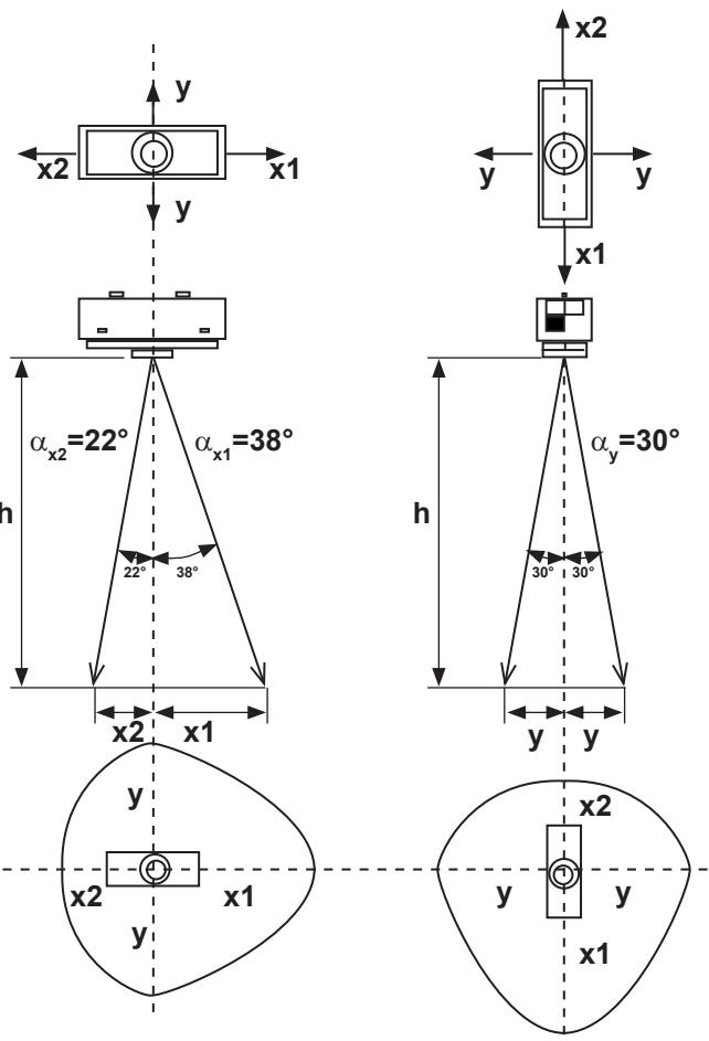
example for light and motion detection area at height of 2,3m.
