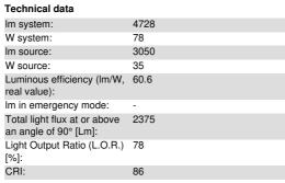
Colour temperature [K]: 6500 Ballast losses [W]: 8 Voltage [Vin]: 230 Lamp code: L105 Socket: G5 Number of lamps for optical 2 assembly: ZVEI Code: T 16 Number of optical assemblies: DALI Control:
