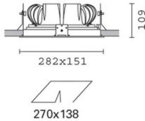
**Product code**MP24: rectangular recessed luminaire with 2 optical assemblies - warm white passive dissipation LEDs - integrated DALI control gear - medium **Attention! Code no longer in production****Technical description**
