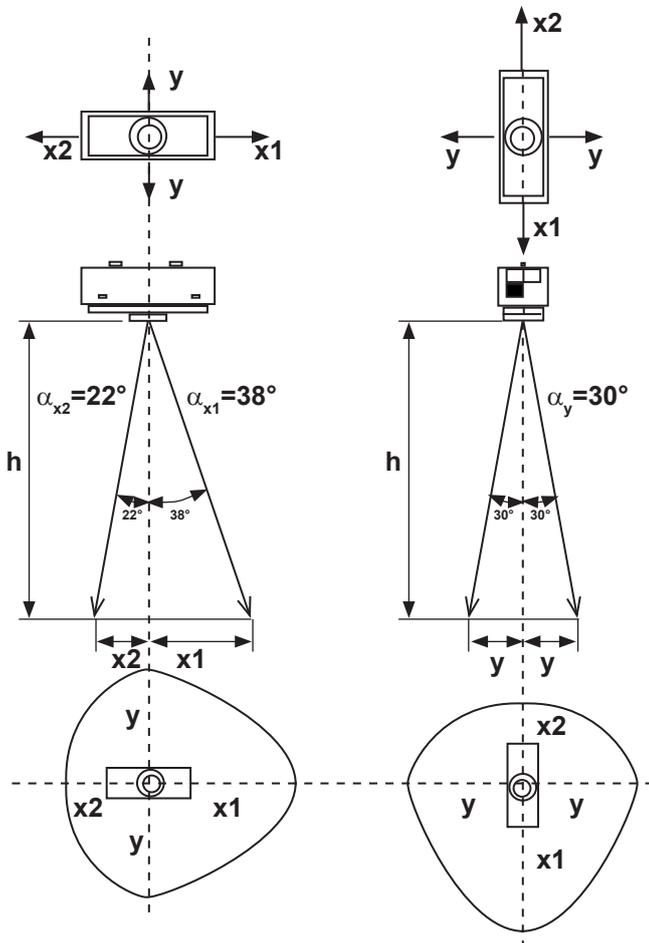
example for light and motion detection area at height of 2,3m.
